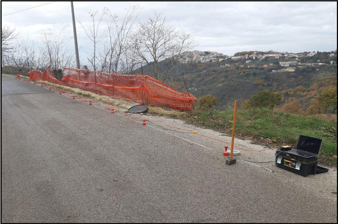
PROVA SISMICA MASW
